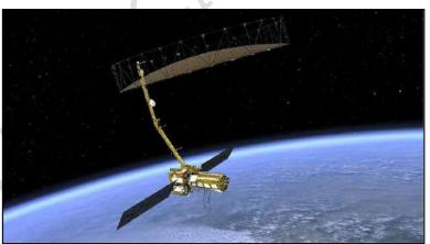
*L-band* (25-centimeter wavelength) detects larger features like tree trunks and penetrates vegetation, while S-band (10-centimeter wavelength) detects smaller features like leaves and rough surfaces.
