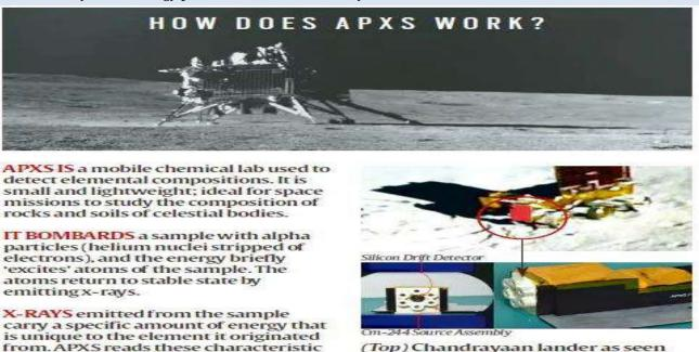
EMISSION RATE of x-rays provides clues about the concentration of a particular element in the sample. Computers on APXS process the data
